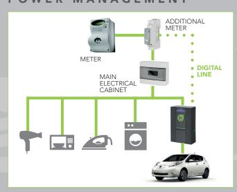
The Wall Box BE-W POWER MANAGEMENT version is a wall charging station compliant with "MODE 3" in accordance with the International Standard IEC/EN 61851-1. Made in halogen-free engineering plastics, it is characterised by a Dual Feel Sensitive finish and a design that highlights its clean and essential lines.
